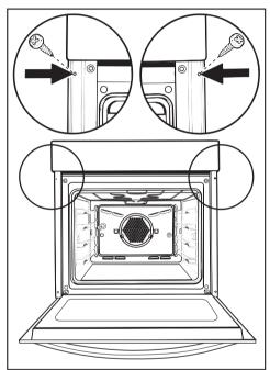
Open the oven door and using two screws secure the oven to the side walls of the housing unit through the holes in the oven trim.
